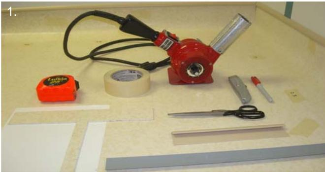
**Tools used:** Heat Gun, Tape measure, utility knife, marking tool, scissors, Tile -T, cove cap, cove stick, masking tape 1-1/2", adhesive brush, chalk line, typing paper, tile cutter.
