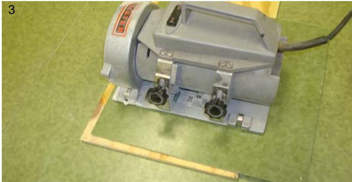
Do a test cut on the tile to check the depth of your router tool on a sample piece of tile. Hold securely in case the depth is set too low.
