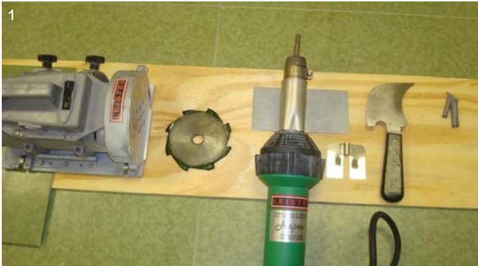
These are the basic tools needed for seam welding, from the left a leister router and replacement blade, leister hot air welding tool. Height guide plate, spatula knife and 4mm bead nozzle.
