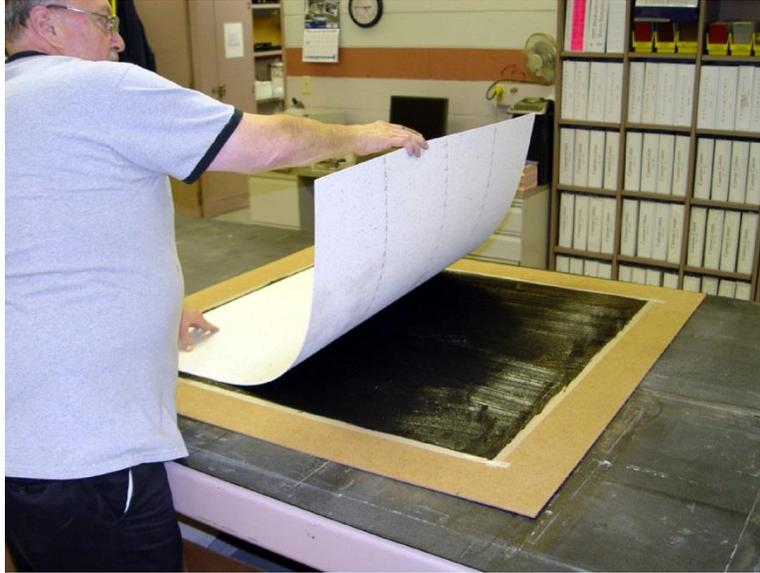
Figure I. Test Floor Preparation - #150 Adhesive
